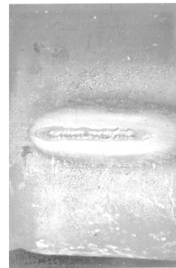
Figure C.4 — Arc or torch burns
